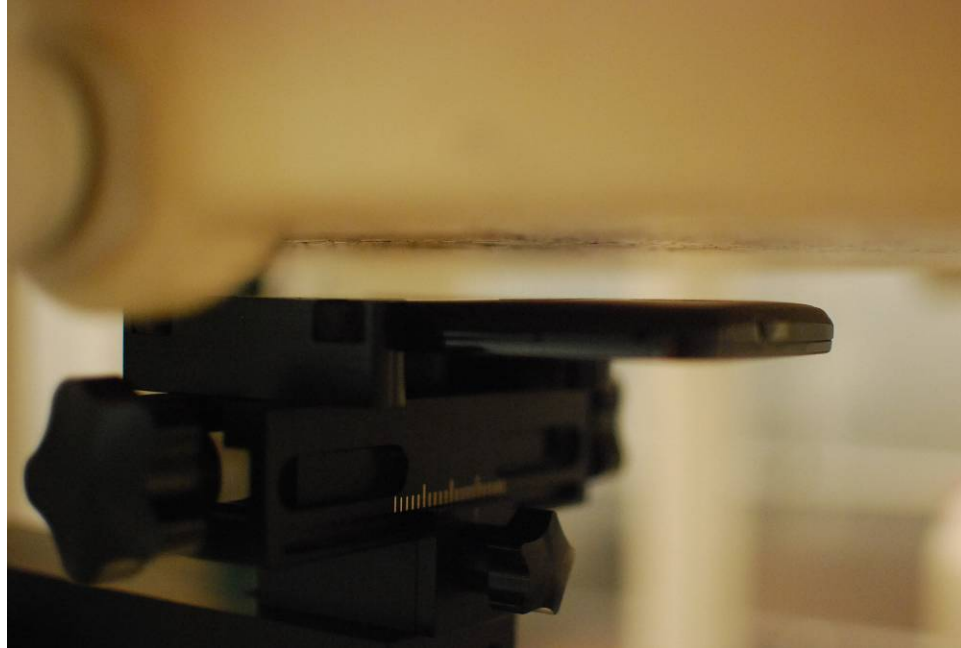
SAR Test Setup Photo 5 – Back at 1.0 cm
