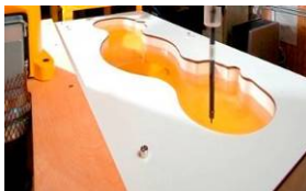
Figure 6-2 SAM Phantom with Simulating Tissue
