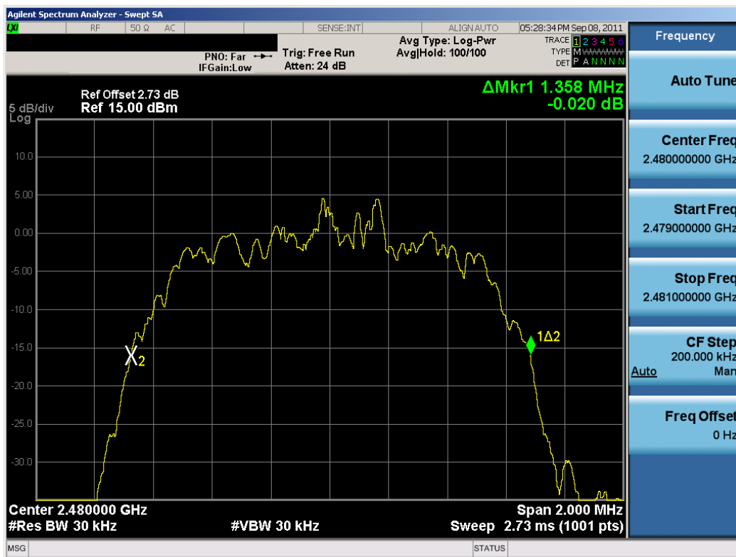
Plot 6-6. 20dB Bandwidth Plot (Bluetooth, 2Mbps – Ch. 78)
