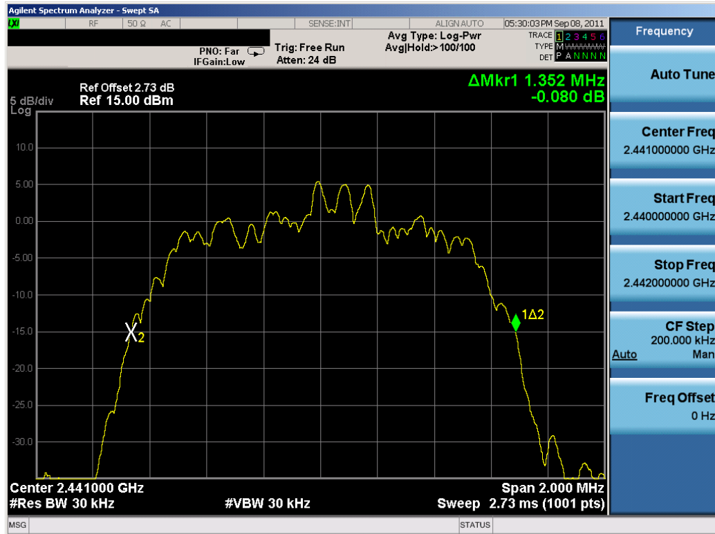
Plot 6-5. 20dB Bandwidth Plot (Bluetooth, 2Mbps – Ch. 39)
