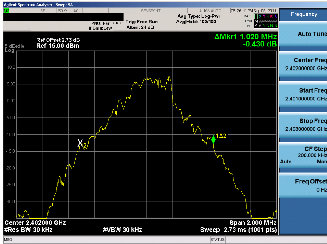
Plot 6-1. 20dB Bandwidth Plot (Bluetooth, 1Mbps – Ch. 0)
