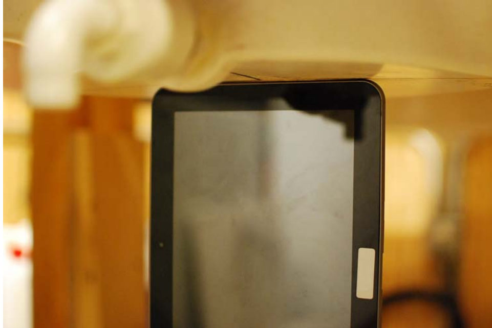
SAR Test Setup Photo 5: Right at 0.0 cm
