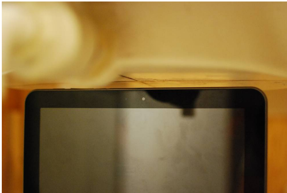
SAR Test Setup Photo 4: Top at 0.5 cm
