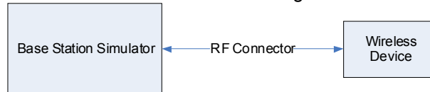
Figure 10-1 Power Measurement Setup
