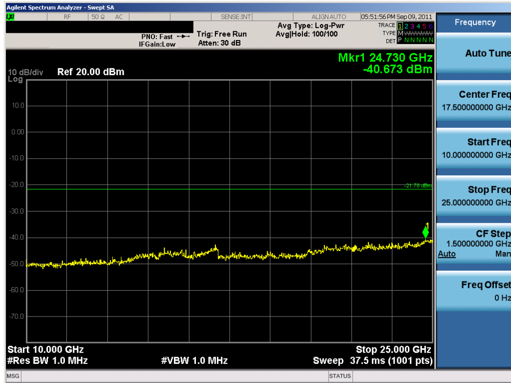
Plot 6-42. Conducted Spurious Plot (802.11b – Ch. 1)
