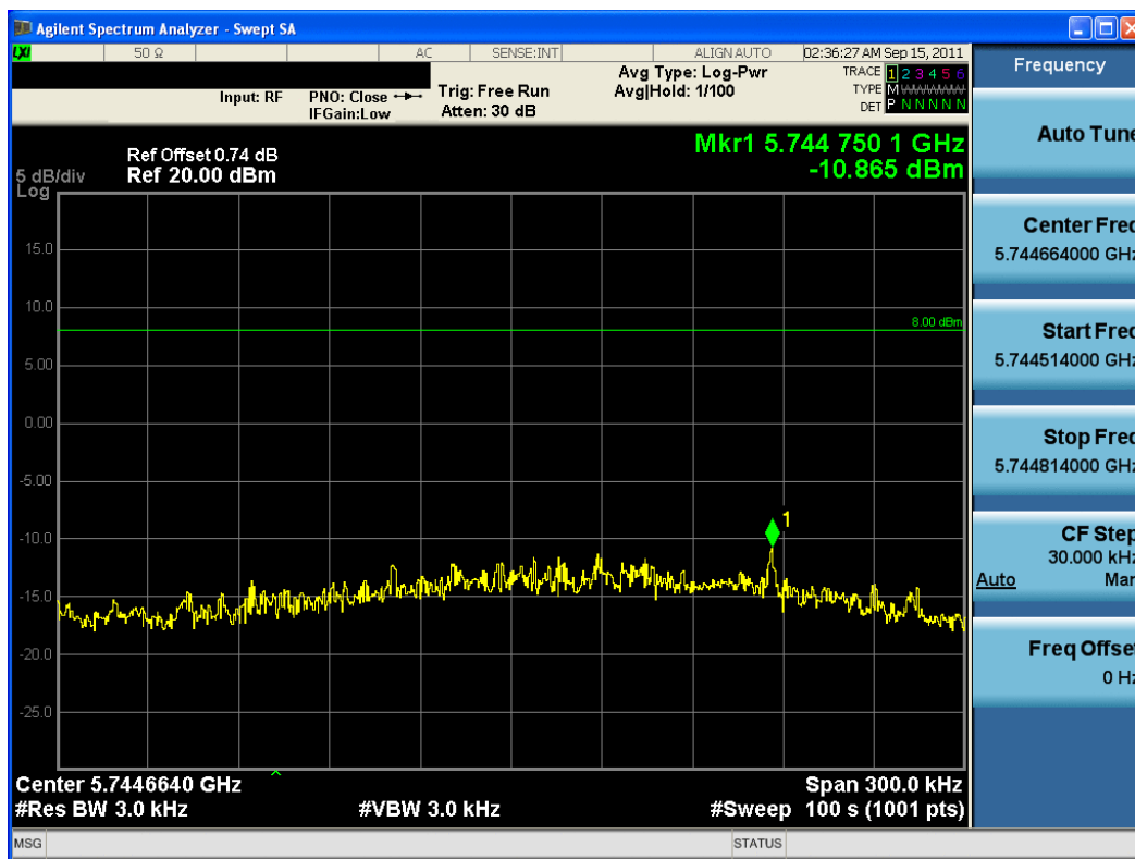
Plot 6-28. Power Spectral Density Plot (802.11n (5.8GHz) – Ch. 149)
