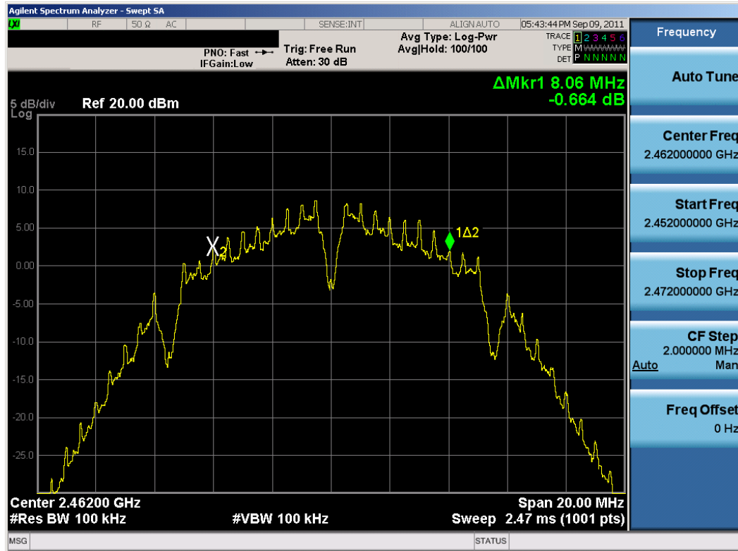
Plot 6-3. 6dB Bandwidth Plot (802.11b – Ch. 11)
