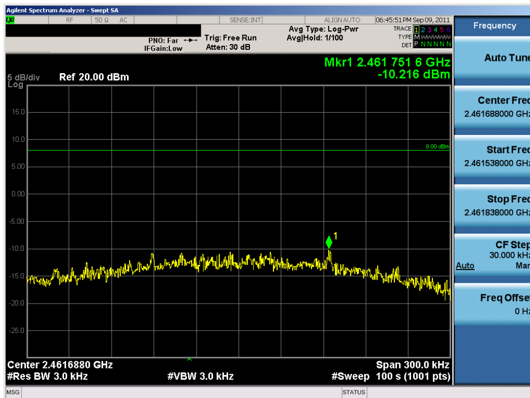
Plot 6-24. Power Spectral Density Plot (802.11n (2.4GHz) – Ch. 11)
