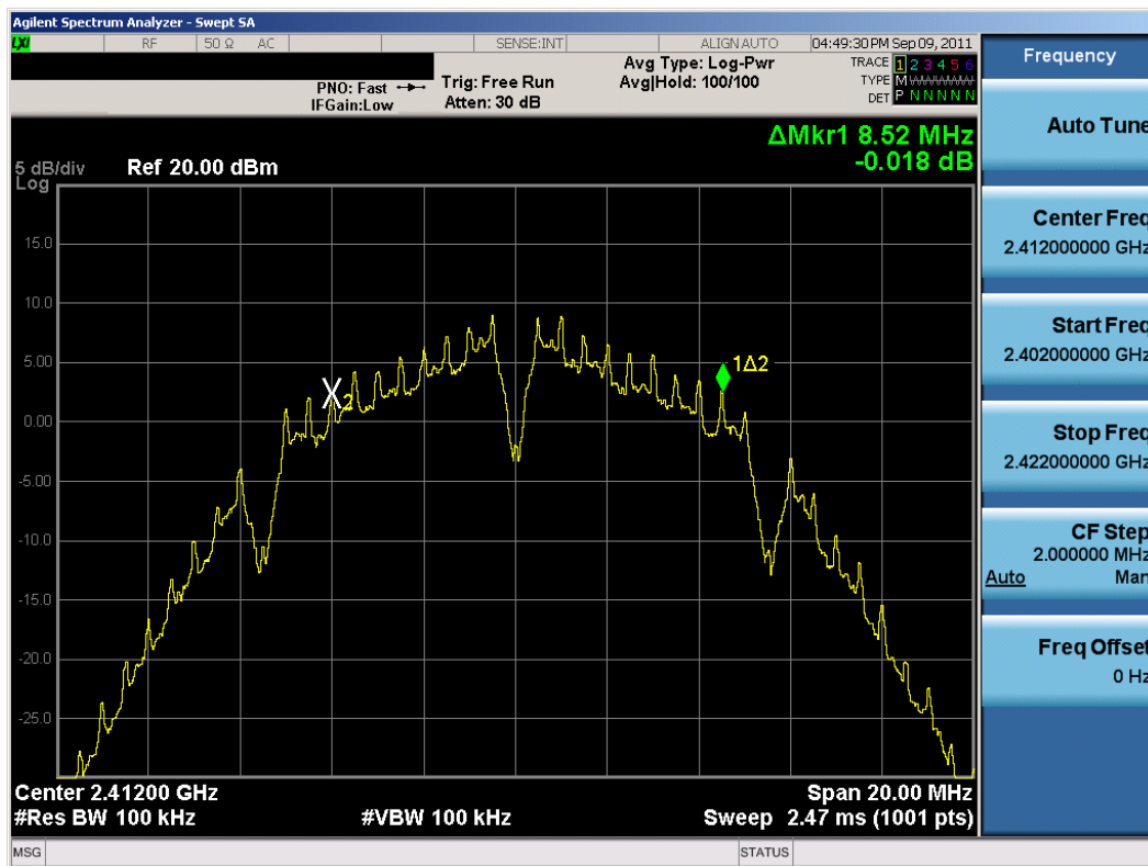
Plot 6-1. 6dB Bandwidth Plot (802.11b – Ch. 1)
