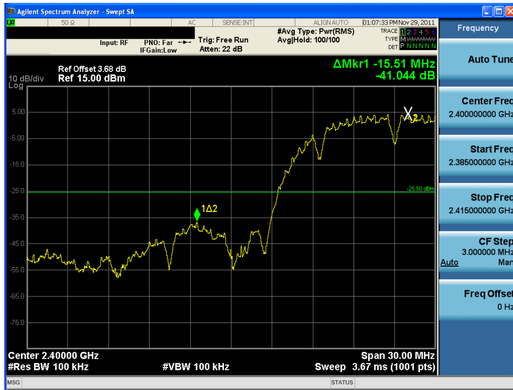
Plot 6-31. Band Edge Plot (802.11b – Ch. 1)
