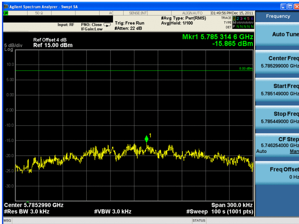
Plot 6-29. Power Spectral Density Plot (802.11n (5.8GHz) – Ch. 157)
