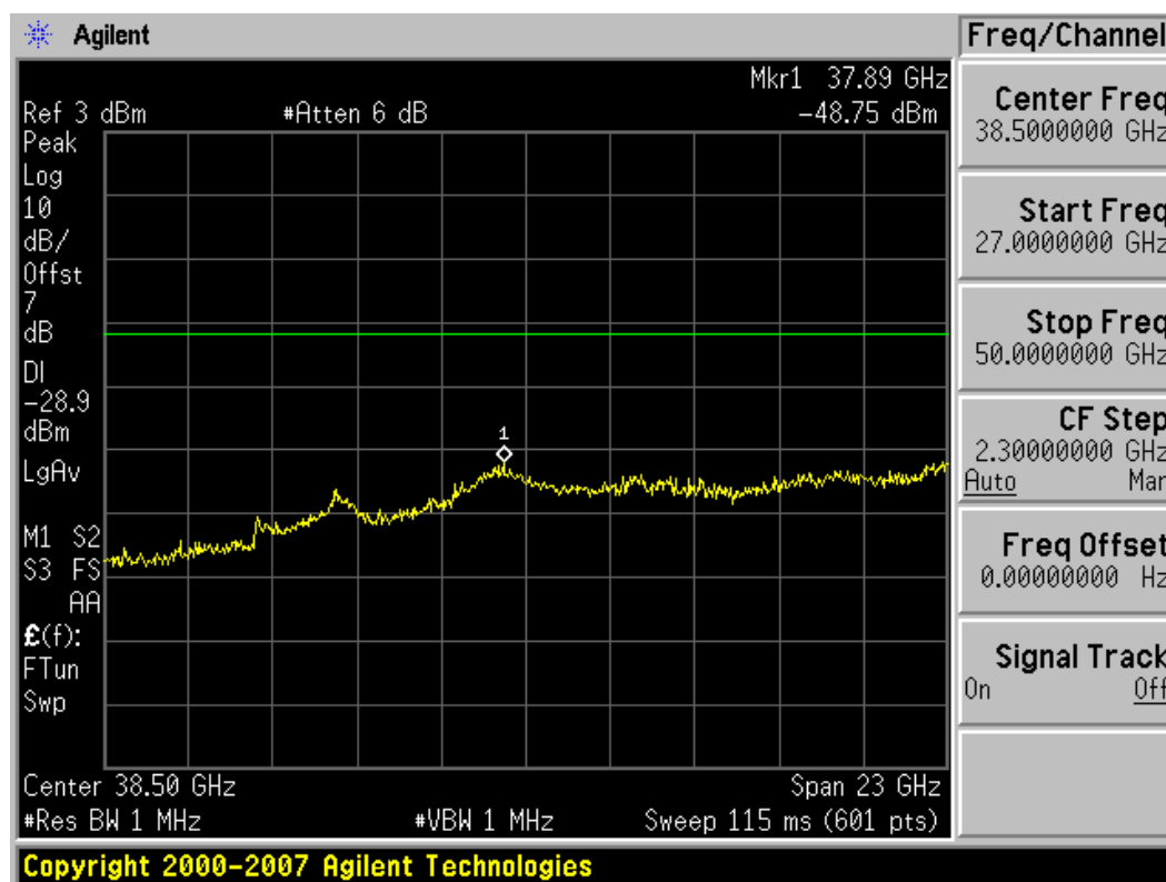
Plot 6-49. Conducted Spurious Plot (802.11a – Ch. 149)
