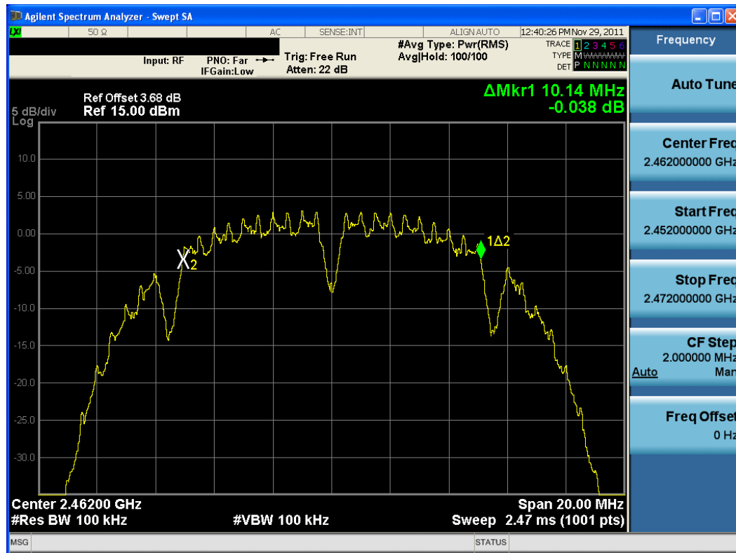
Plot 6-3. 6dB Bandwidth Plot (802.11b – Ch. 11)
