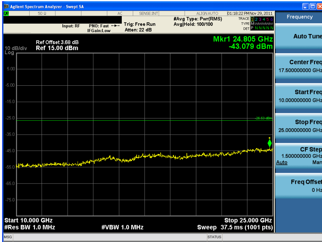
Plot 6-44. Conducted Spurious Plot (802.11b – Ch. 6)
