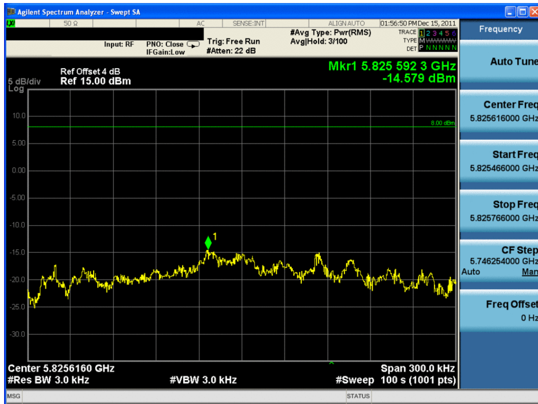
Plot 6-30. Power Spectral Density Plot (802.11n (5.8GHz) – Ch. 165)
