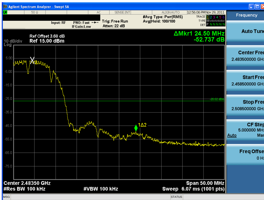
Plot 6-32. Band Edge Plot (802.11b – Ch. 11)
