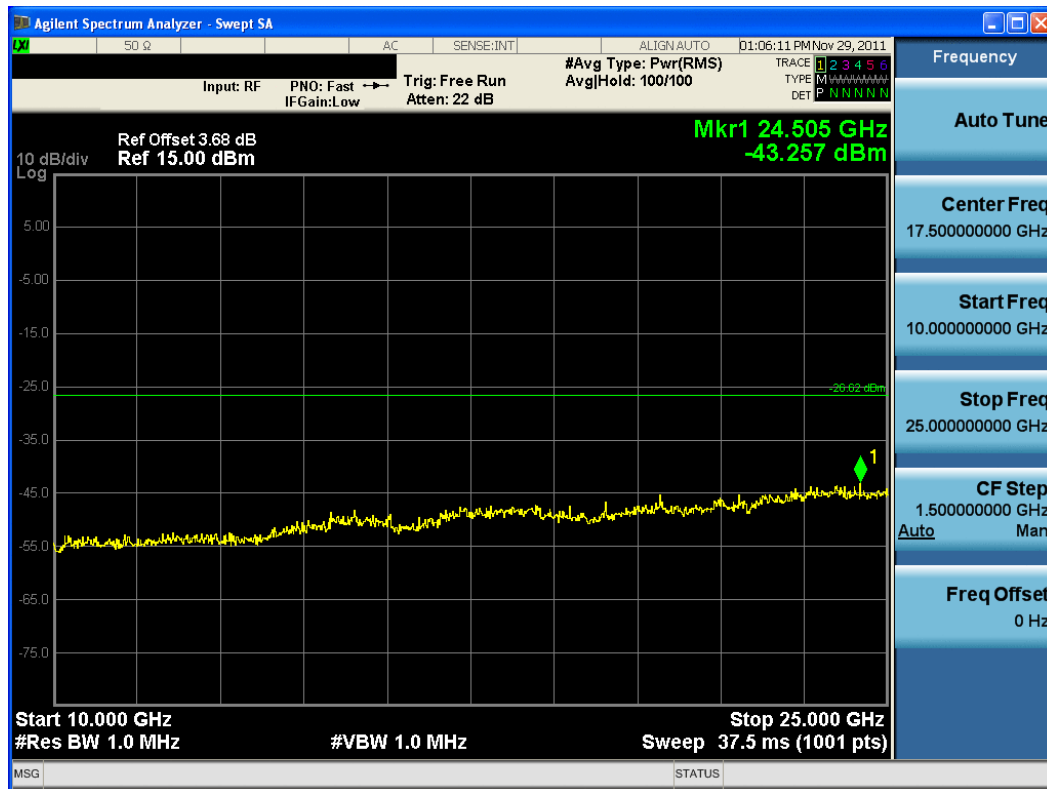
Plot 6-46. Conducted Spurious Plot (802.11b – Ch. 11)
