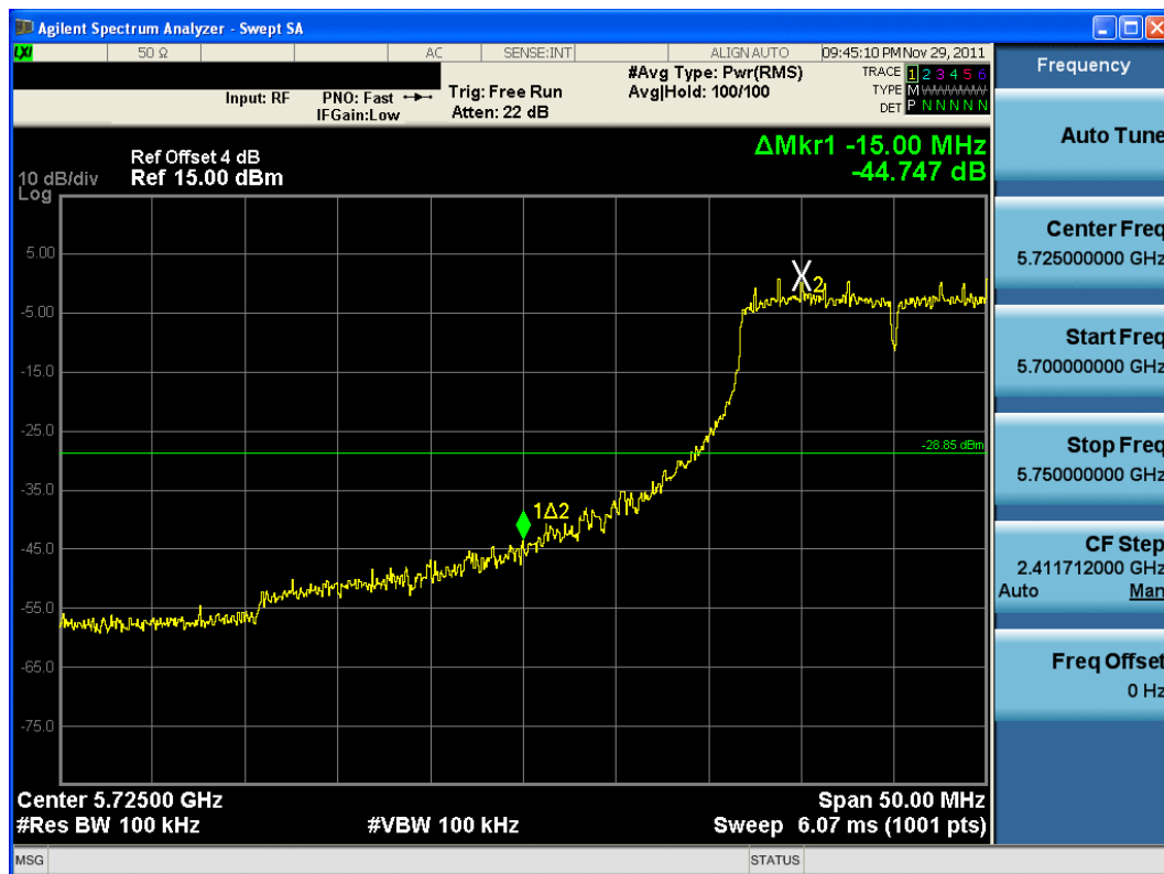
Plot 6-37. Band Edge Plot (802.11a – Ch. 149)
