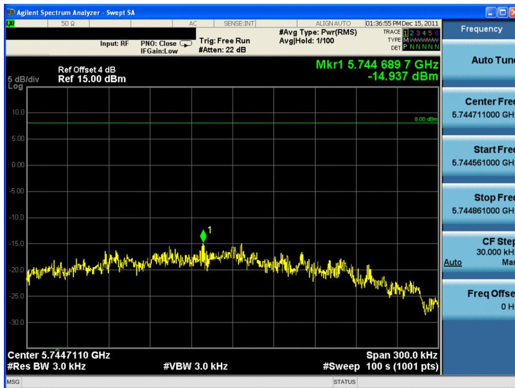
Plot 6-25. Power Spectral Density Plot (802.11a – Ch. 149)
