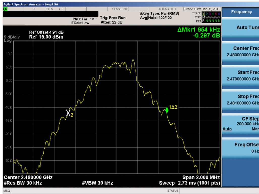
Plot 6-3. 20dB Bandwidth Plot (Bluetooth, 1Mbps – Ch. 78)
