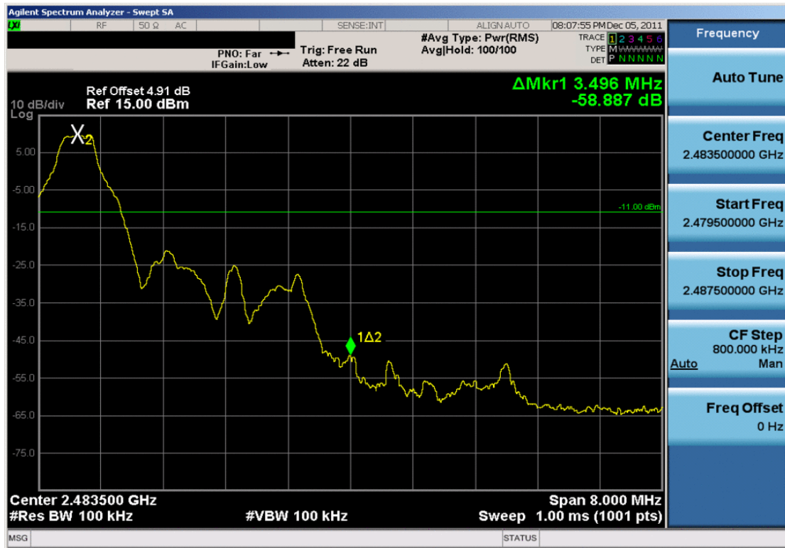
Plot 6-11. Band Edge Plot (Bluetooth, 1Mbps - Ch. 78)
