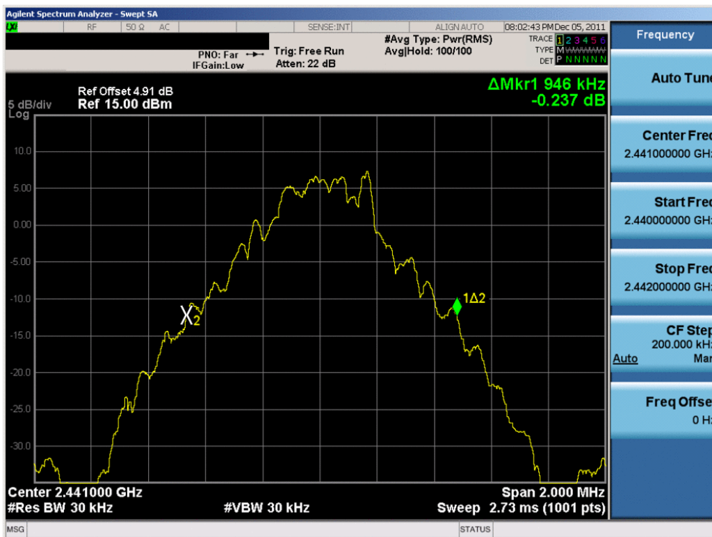
Plot 6-2. 20dB Bandwidth Plot (Bluetooth, 1Mbps – Ch. 39)
