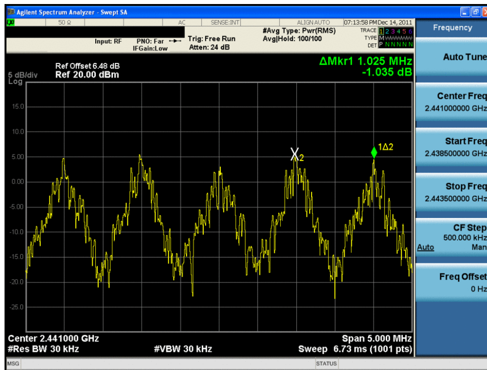
Plot 6-12. Channel Spacing Plot (Bluetooth)
