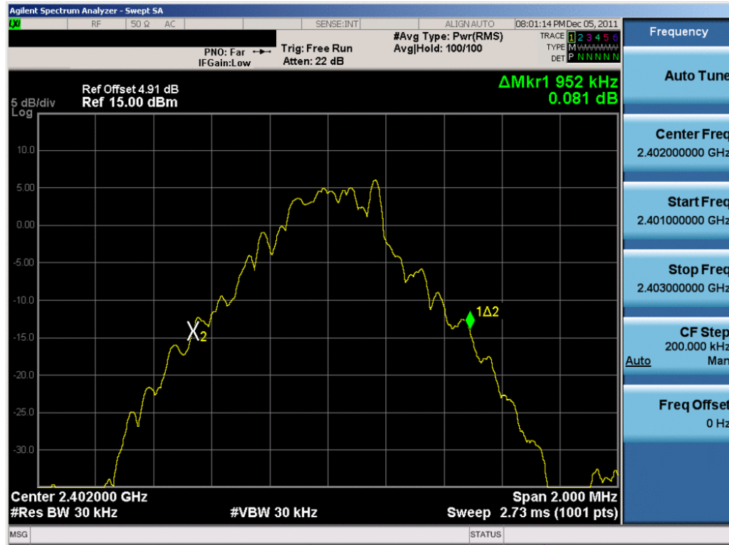
Plot 6-1. 20dB Bandwidth Plot (Bluetooth, 1Mbps – Ch. 0)
