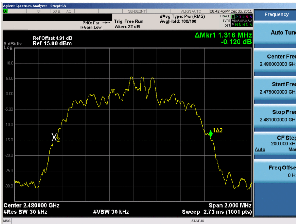
Plot 6-6. 20dB Bandwidth Plot (Bluetooth, 2Mbps – Ch. 78)
