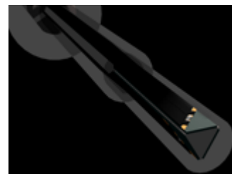
Figure 4-3 Triangular Probe Configuration
