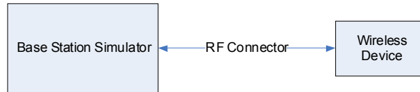
Figure 11-1 Power Measurement Setup
