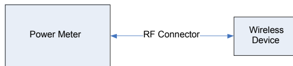
Figure 12-1 Power Measurement Setup
