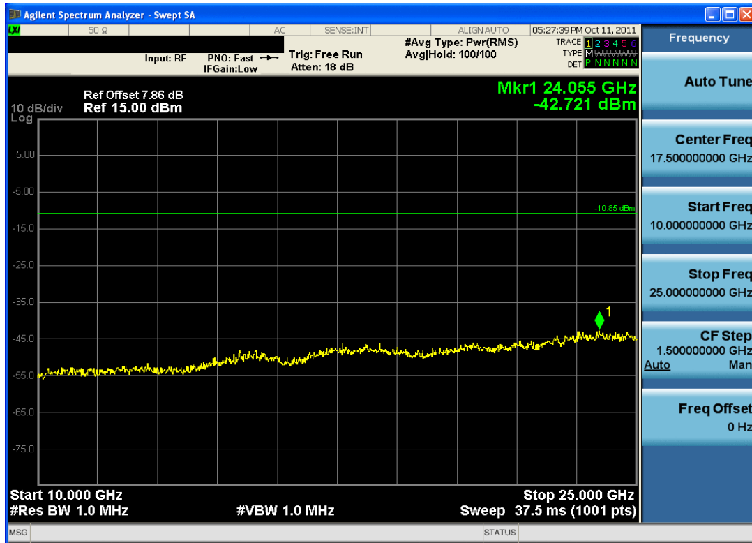
Plot 6-19. Conducted Spurious Plot (Bluetooth, 2Mbps – Ch. 39)
