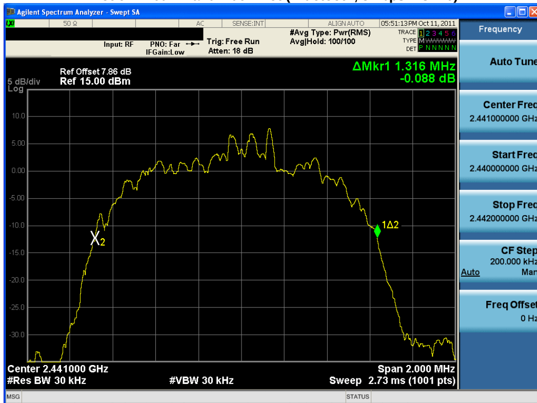
Plot 6-8. 20dB Bandwidth Plot (Bluetooth, 3Mbps - Ch. 39)
