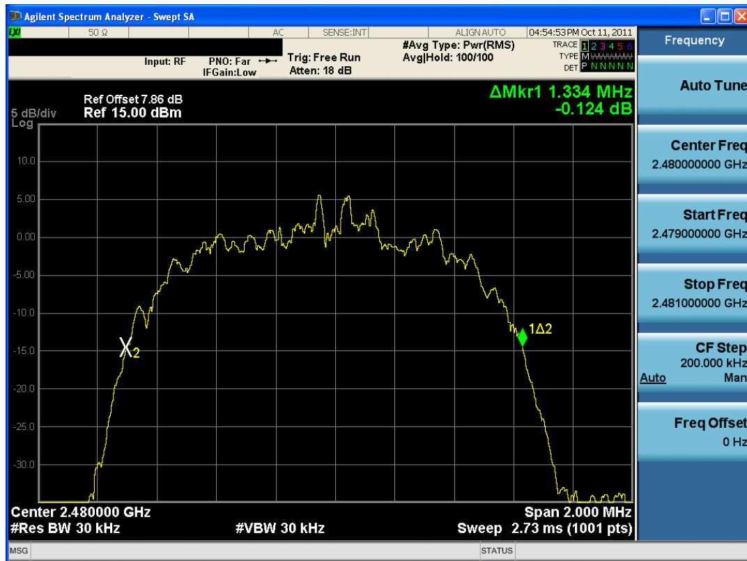
Plot 6-9. 20dB Bandwidth Plot (Bluetooth, 3Mbps – Ch. 78)
