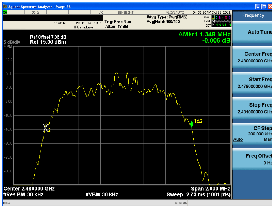
Plot 6-6. 20dB Bandwidth Plot (Bluetooth, 2Mbps – Ch. 78)
