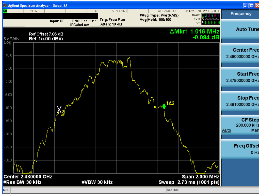
Plot 6-3. 20dB Bandwidth Plot (Bluetooth, 1Mbps – Ch. 78)
