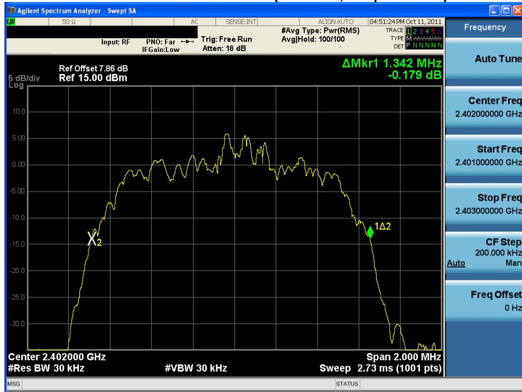
Plot 6-4. 20dB Bandwidth Plot (Bluetooth, 2Mbps – Ch. 0)
