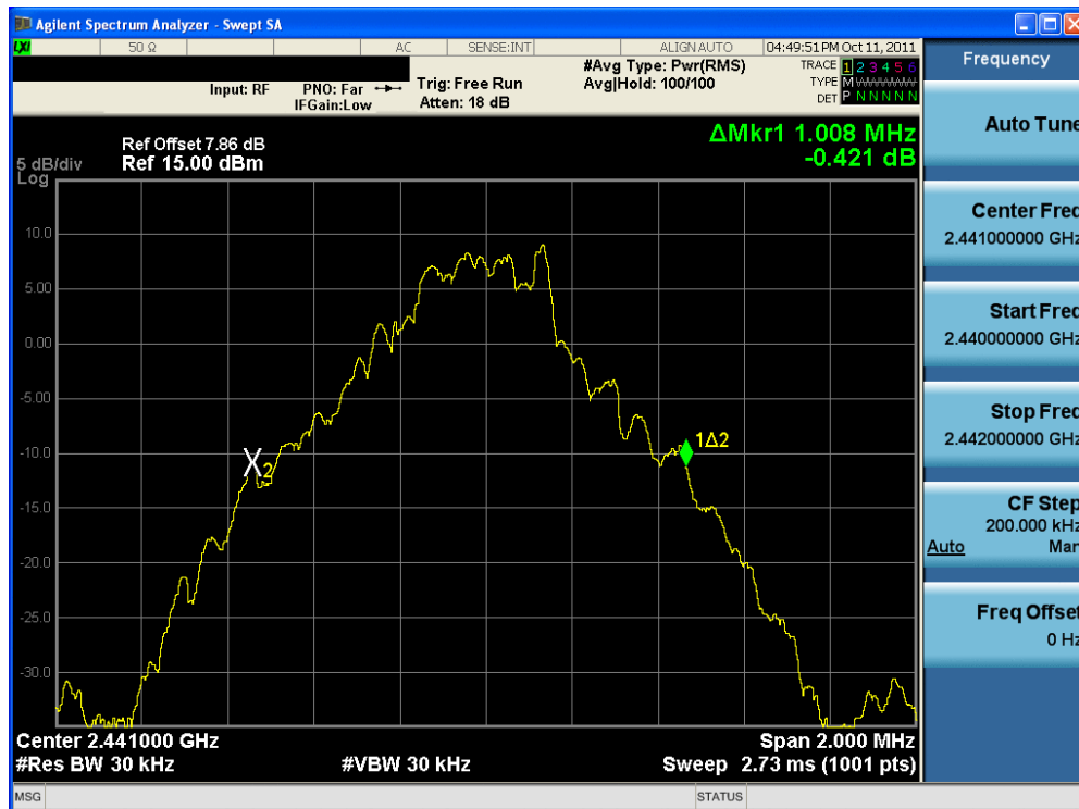
Plot 6-2. 20dB Bandwidth Plot (Bluetooth, 1Mbps – Ch. 39)
