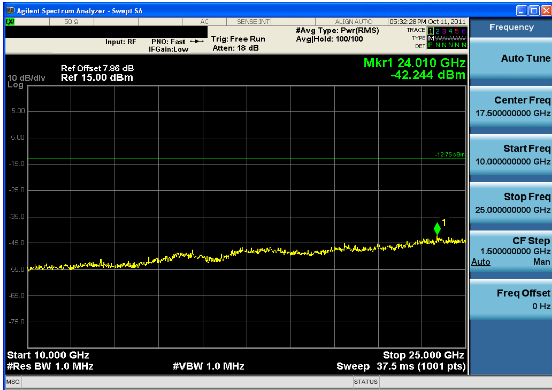
Plot 6-17. Conducted Spurious Plot (Bluetooth, 2Mbps – Ch. 0)
