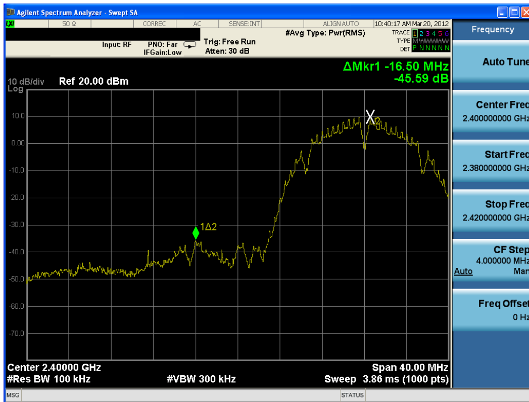
Plot 6-31. Band Edge Plot (802.11b – Ch. 1)
