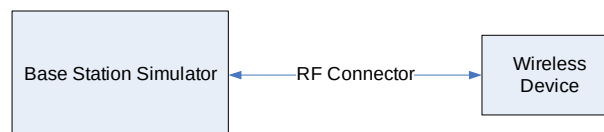
Figure 9-1 Power Measurement Setup
