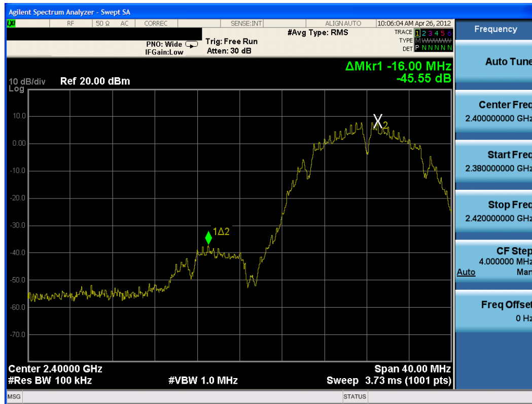
Plot 6-35. Band Edge Plot (802.11b – Ch. 1)
