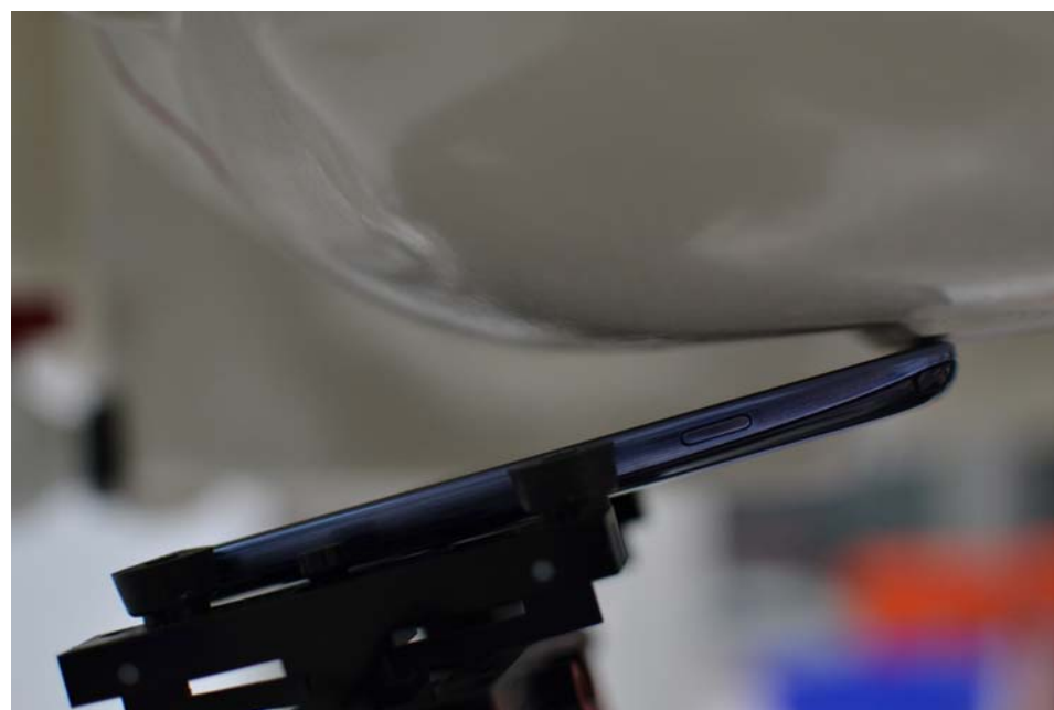
SAR Test Setup Photo 4 – Left Tilt
