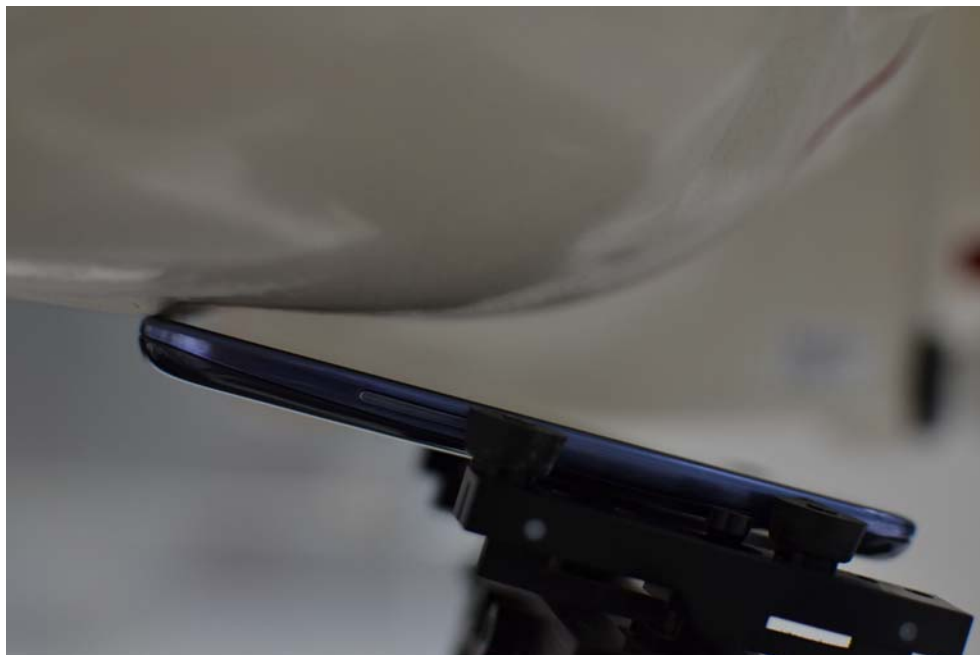
SAR Test Setup Photo 2 – Right Tilt
