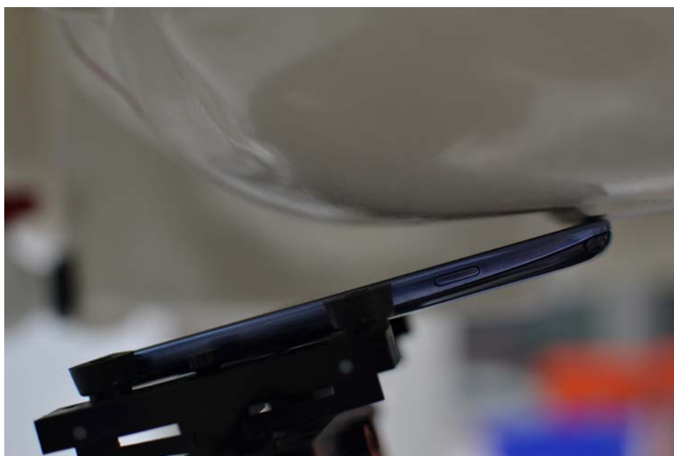
SAR Test Setup Photo 4 – Left Tilt
