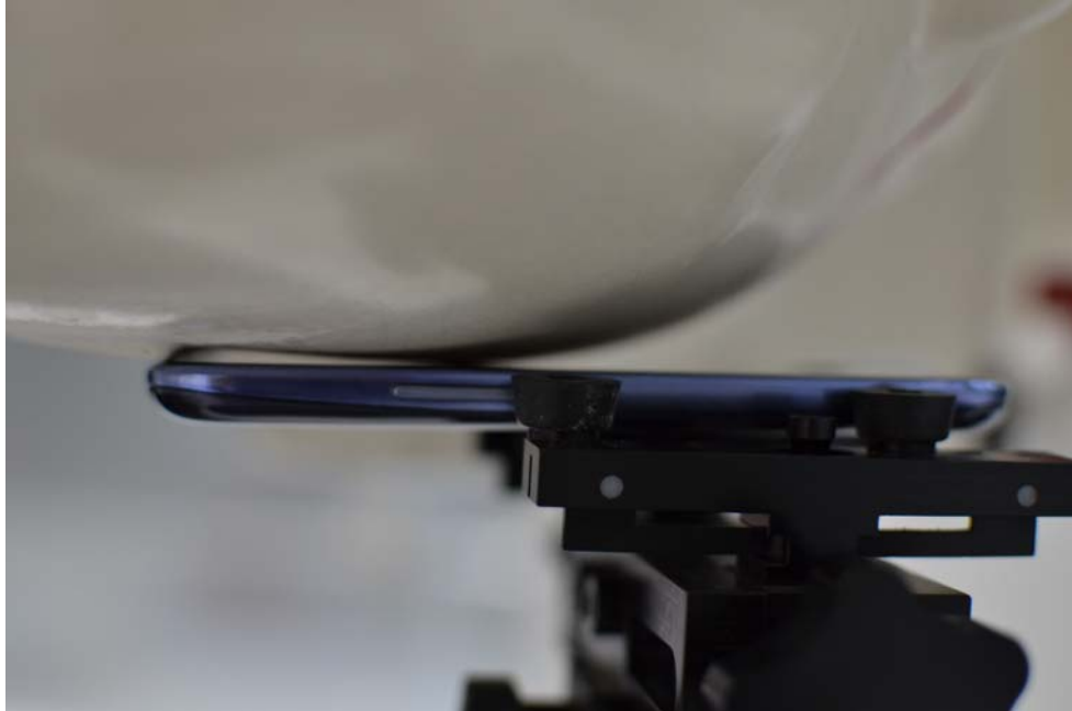
SAR Test Setup Photo 1 – Right Touch
