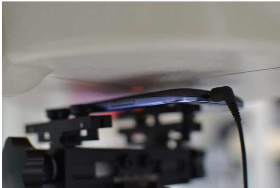
SAR Test Setup Photo 10 – Body-Worn Back Side at 1.0 cm
