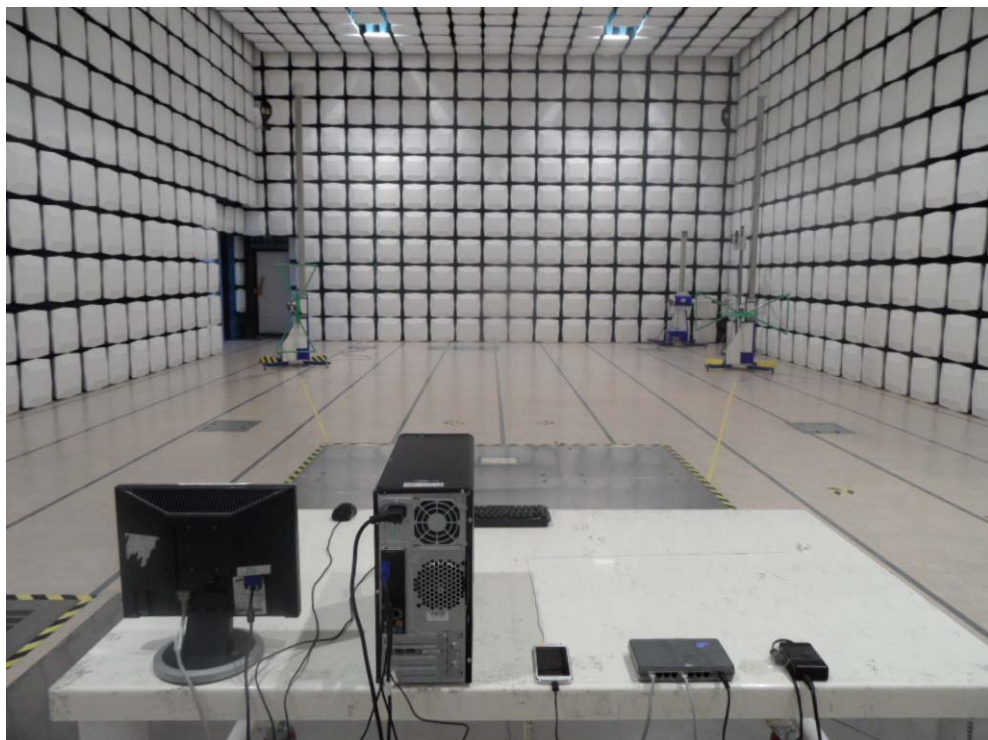
[ Radiated Disturbance for Below 1 GHz – Rear ]
