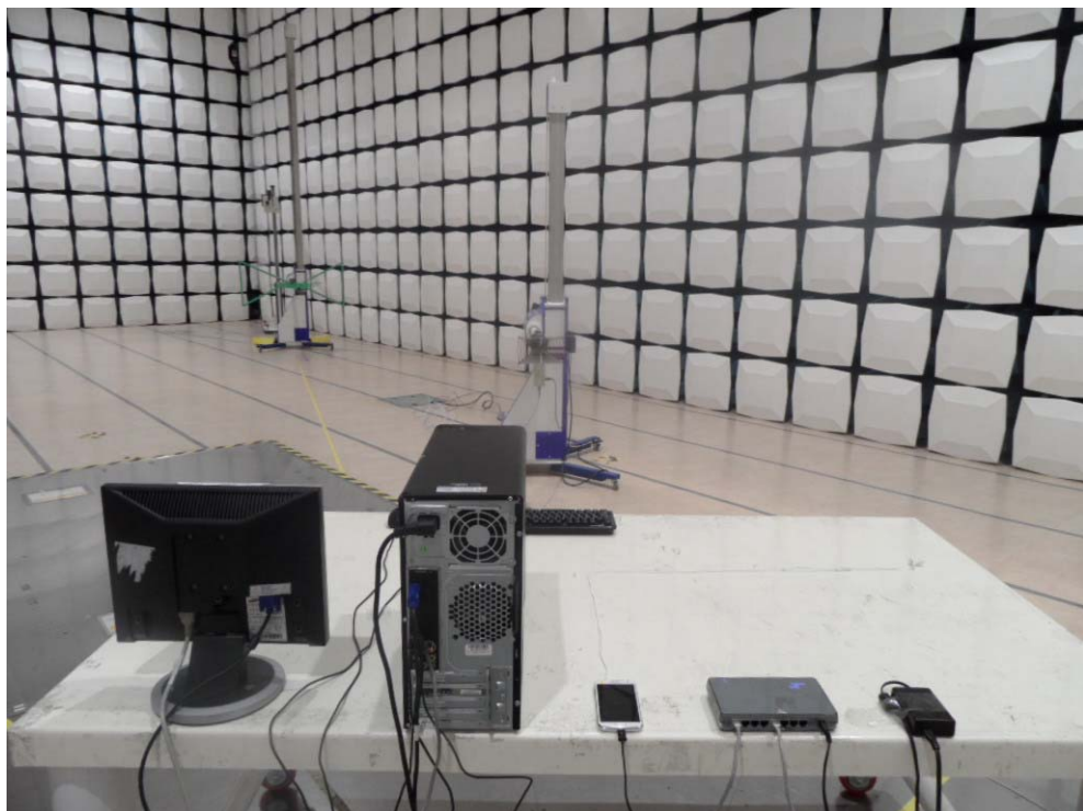
[ Radiated Disturbance for Above 1 GHz – Rear ]
