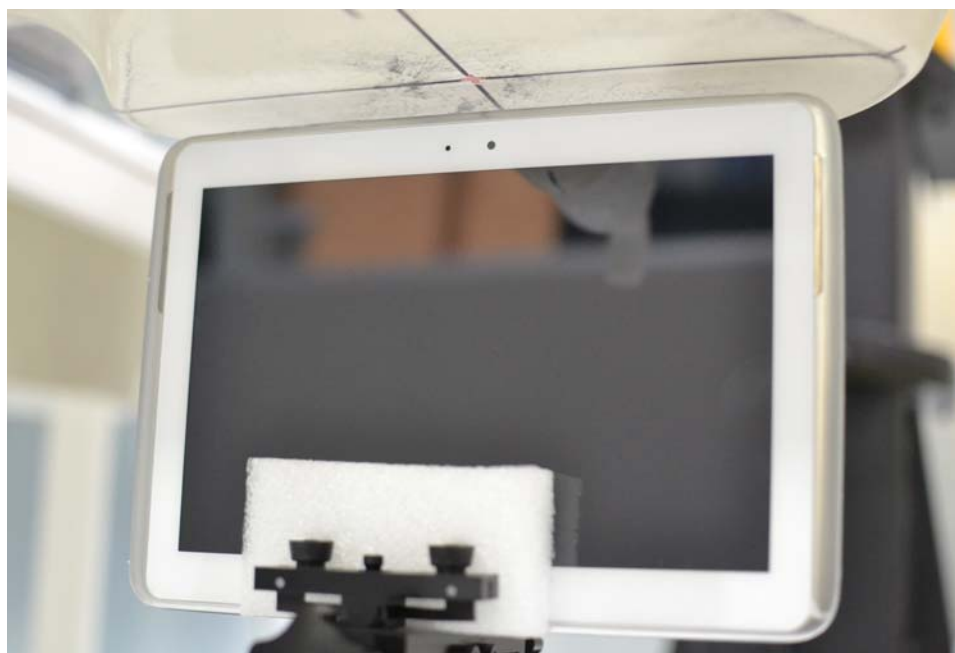
SAR Test Setup Photo 2: Top Edge at 0.9 cm
