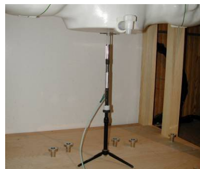
Figure 9-2 System Verification Setup Photo
