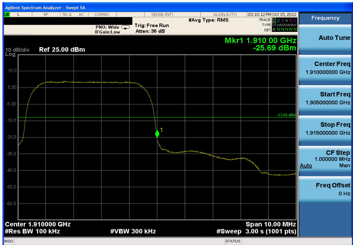
Plot 7-30. Band Edge Plot (PCS WCDMA Mode – Ch. 9538)
