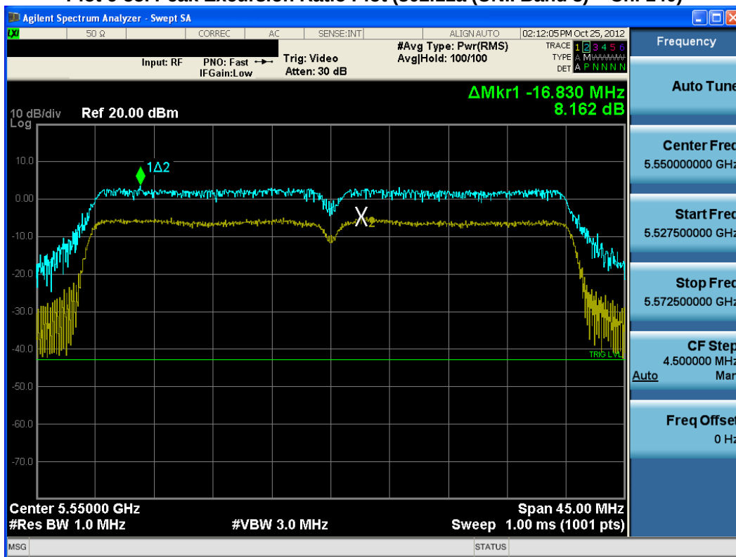
Plot 6-56. Peak Excursion Ratio Plot (40MHz BW 802.11n (UNII Band 3) – Ch. 110)
