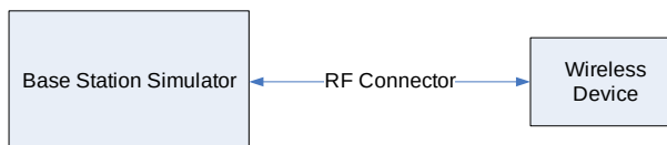
Figure 9-1 Power Measurement Setup
