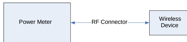
Figure 9-3 Power Measurement Setup
