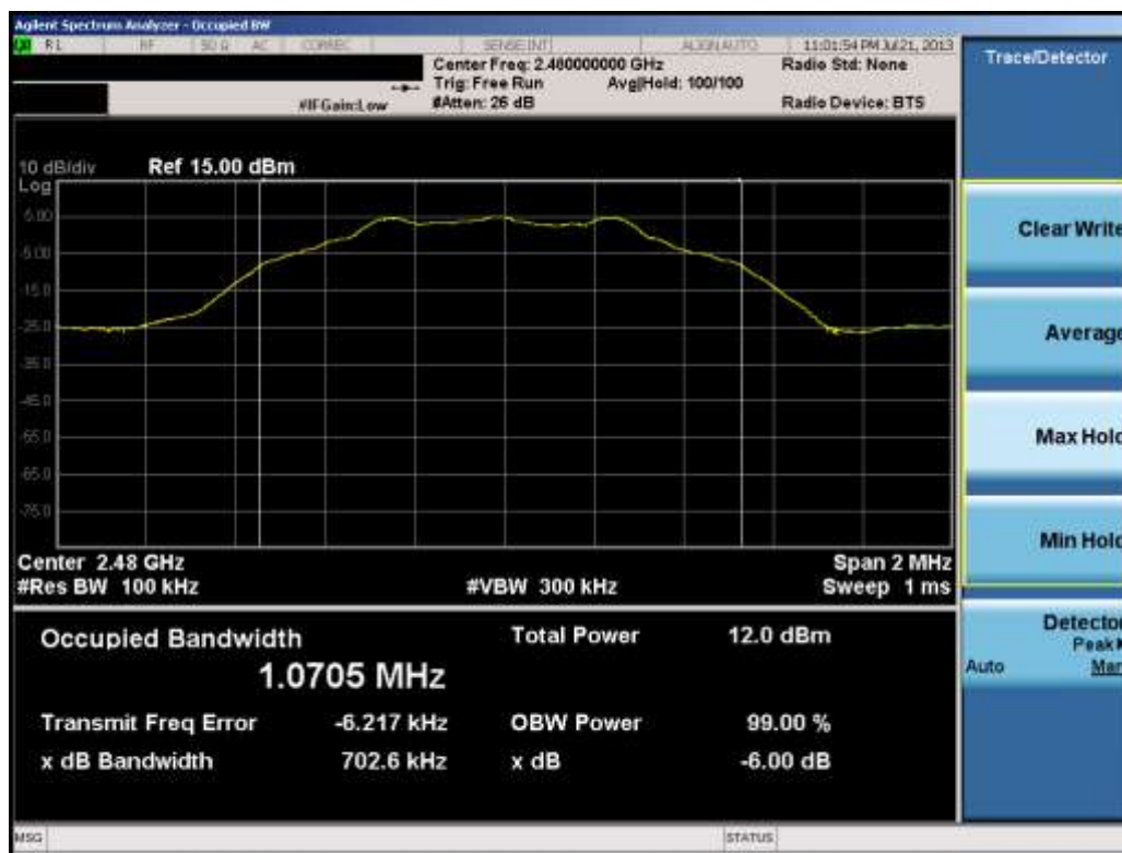
Plot 6-3. 6dB Bandwidth Plot (Bluetooth (LE) – Ch. 39)
