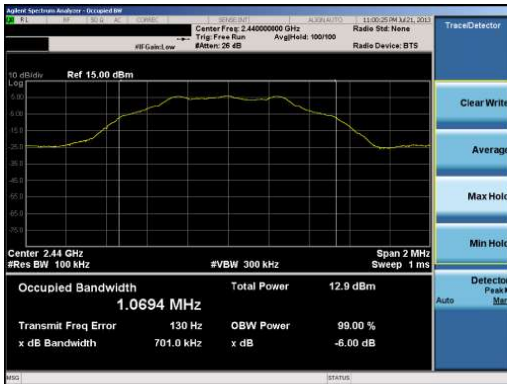
Plot 6-2. 6dB Bandwidth Plot (Bluetooth (LE) – Ch. 19)
