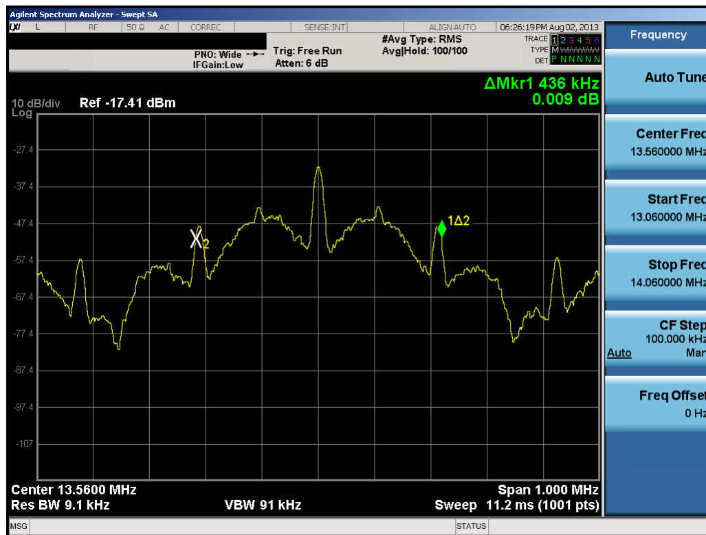
Figure 8-2. 20dB Bandwidth Plot
