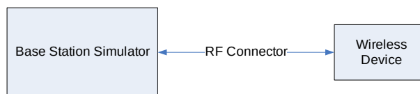
Figure 9-2 Power Measurement Setup
