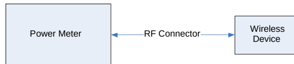
Figure 9-3 Power Measurement Setup
