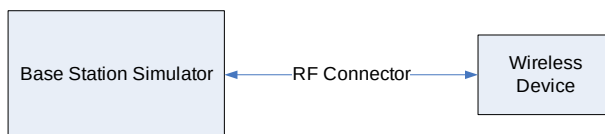
Figure 9-1 Power Measurement Setup
