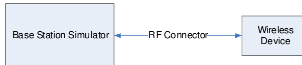
Figure 9-1 Power Measurement Setup
