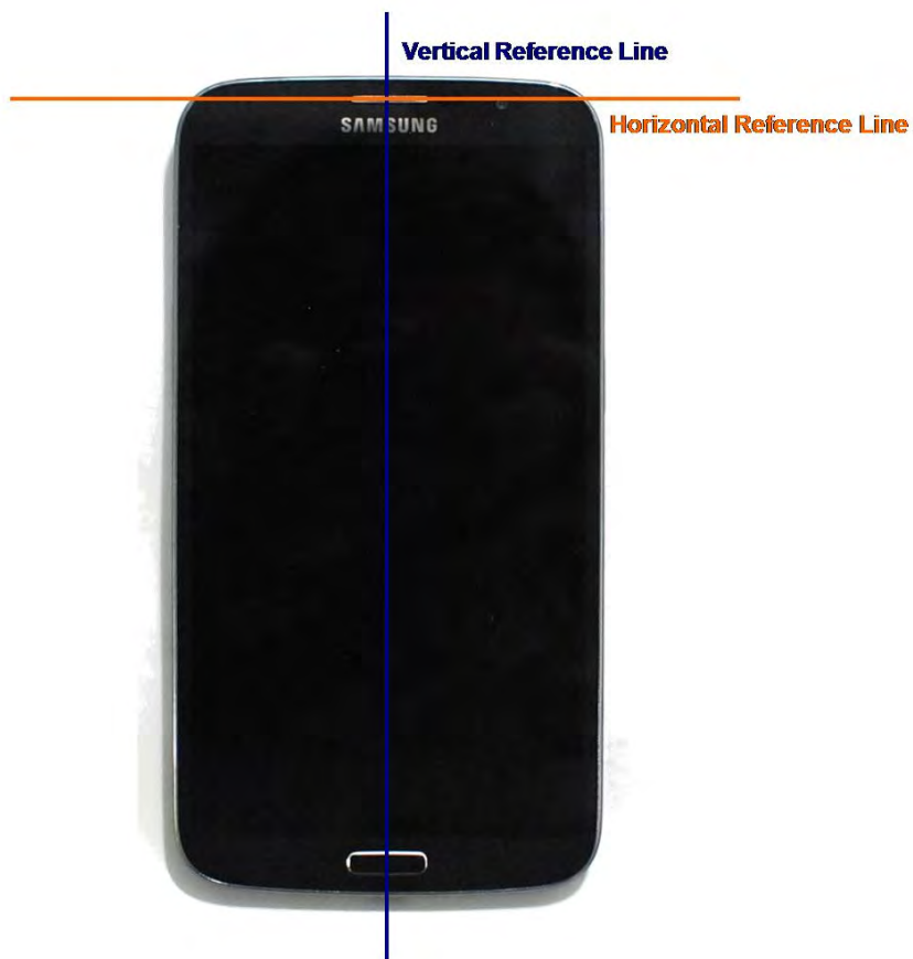
SAR Test Setup Photo 15: Horizontal and Vertical Reference Lines
