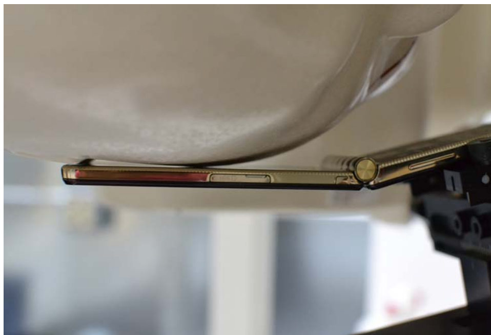
SAR Test Setup Photo 3: Right Cheek
