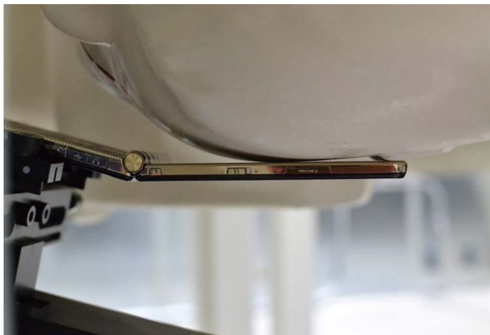
SAR Test Setup Photo 5: Left Cheek
