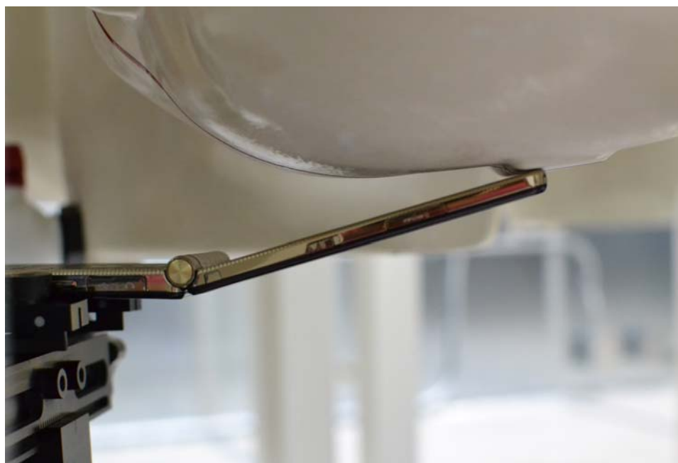
SAR Test Setup Photo 6: Left Tilt
