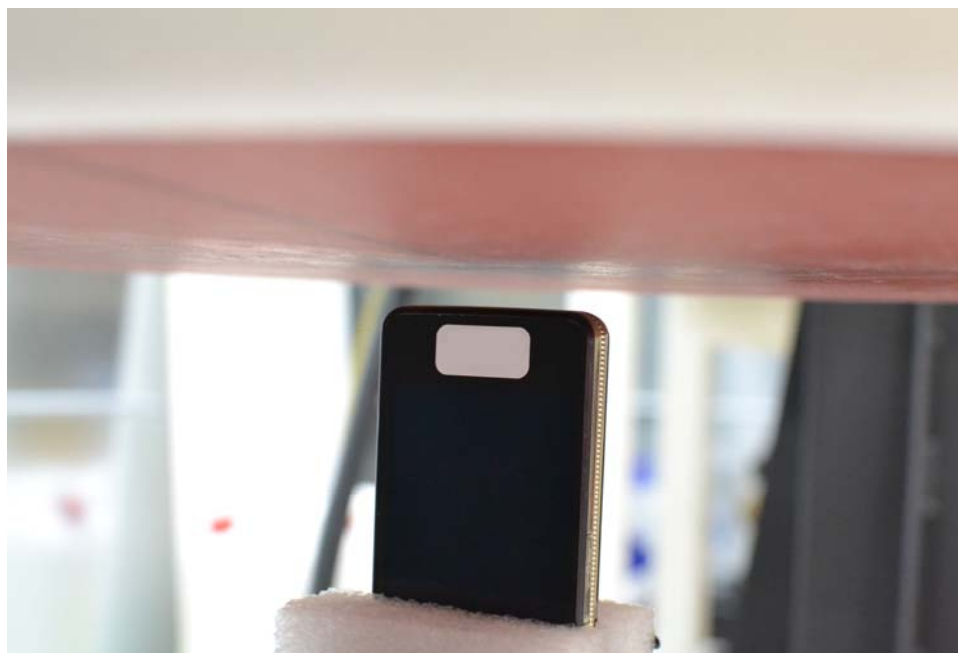
SAR Test Setup Photo 10: Bottom Edge at 1.0 cm
