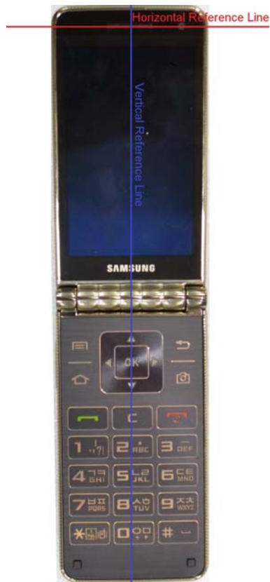
SAR Test Setup Photo 13: Horizontal and Vertical Reference Lines
