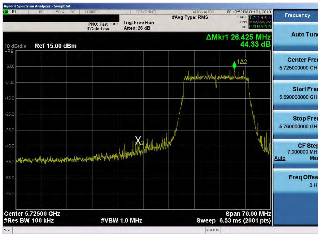
Plot 6-45. Band Edge Plot (20MHz BW 802.11n (5.8GHz) – Ch. 149)
