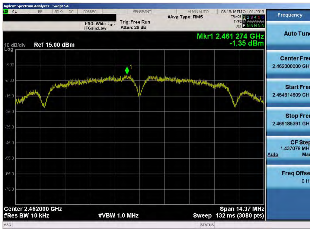
Plot 6-21. Power Spectral Density Plot (802.11b – Ch. 11)
