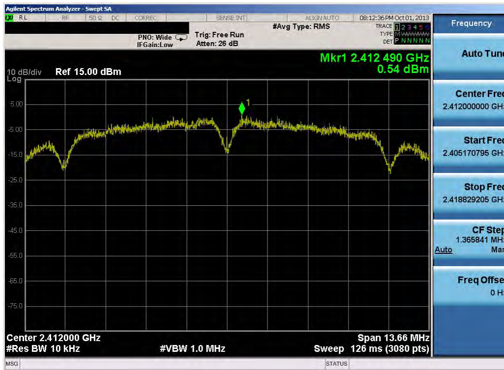
Plot 6-19. Power Spectral Density Plot (802.11b – Ch. 1)
