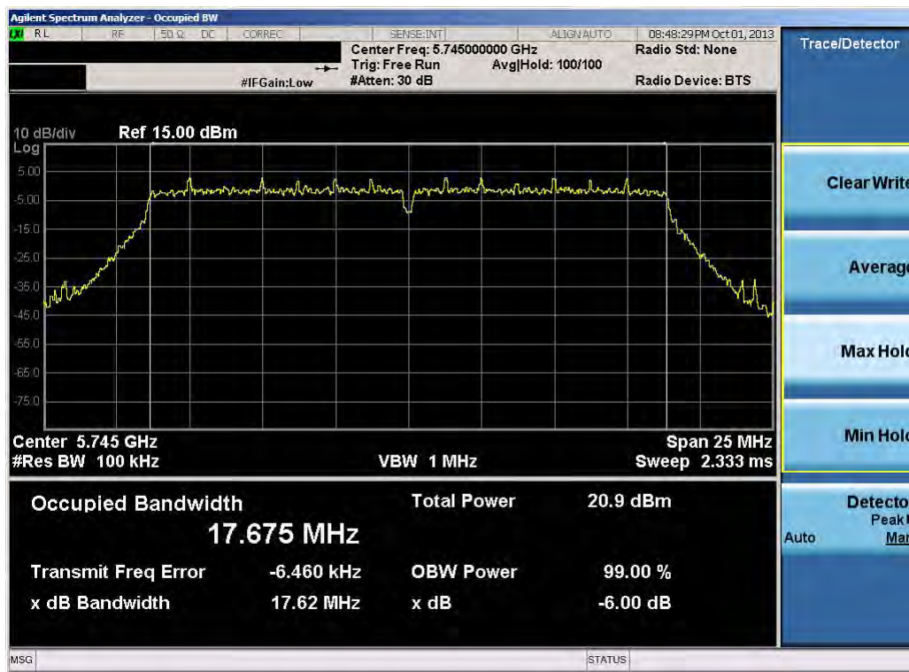
Plot 6-13. 6dB Bandwidth Plot (20MHz BW 802.11n (5.8GHz) – Ch. 149)
