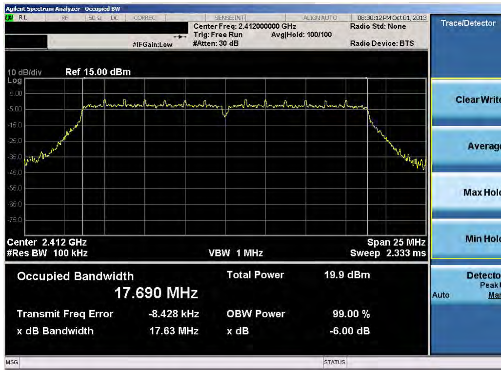
Plot 6-7. 6dB Bandwidth Plot (802.11n (2.4GHz) – Ch. 1)
