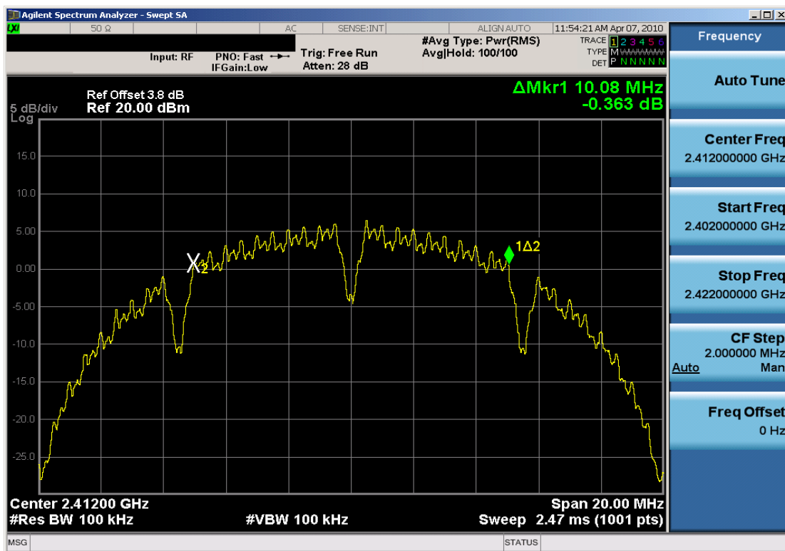
Plot 6-1. 6dB Bandwidth Plot (802.11b – Ch. 1)
