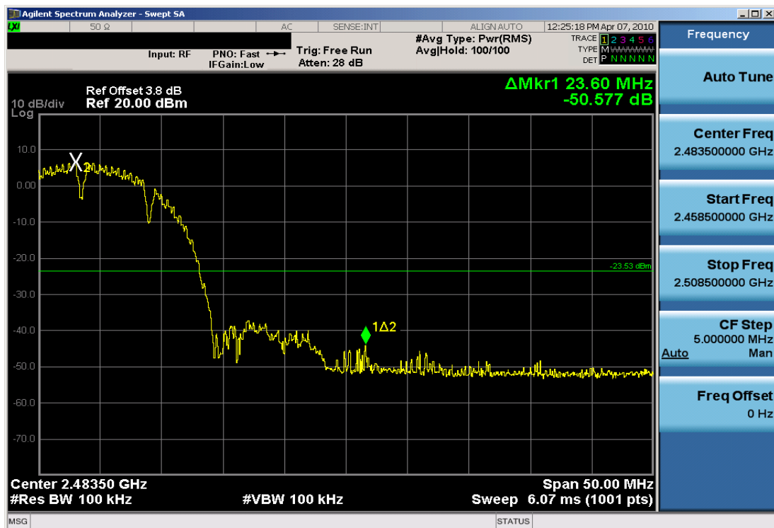
Plot 6-14. Band Edge Plot (802.11b – Ch. 11)
