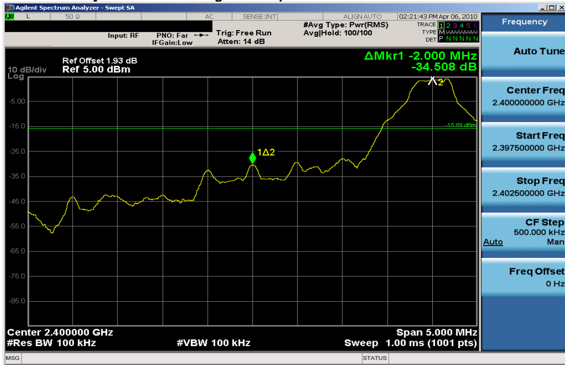
Plot 6-4. Band Edge Plot (Bluetooth – Ch. 0)
