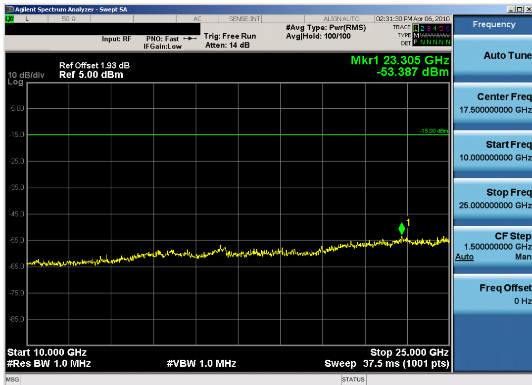
Plot 6-17. Conducted Spurious Plot (Bluetooth – Ch. 78)
