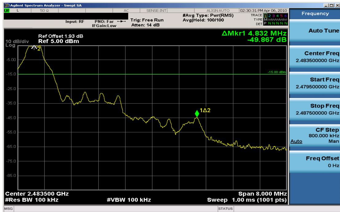
Plot 6-5. Band Edge Plot (Bluetooth – Ch. 78)
