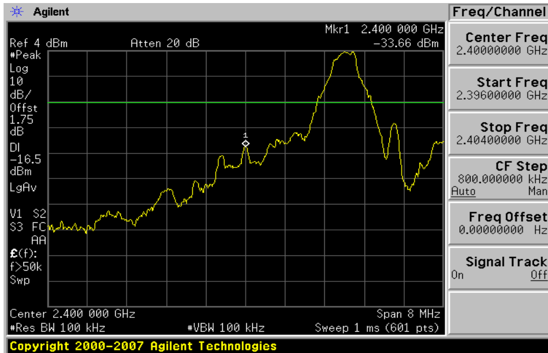
Plot 6-4. Band Edge Plot (Bluetooth – Ch. 0)
