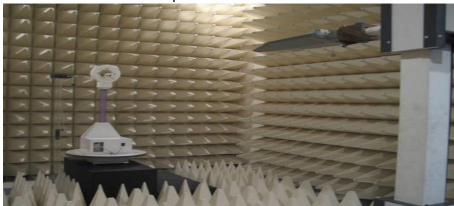
Figure2. Photograph of 3m Fully-Anechoic Chamber
