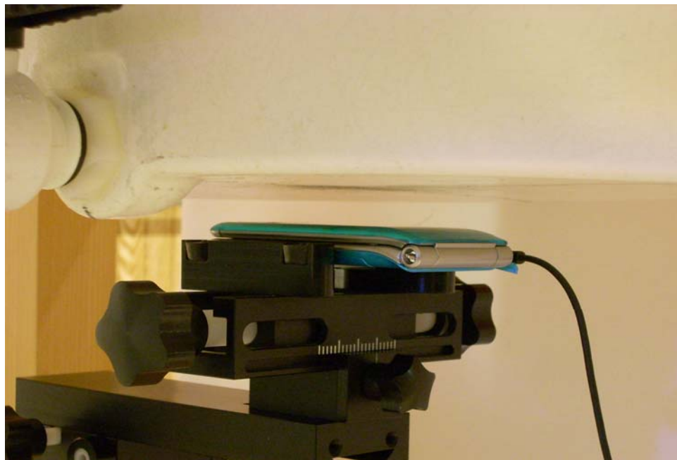
Figure 19-8 SAR Test Setup Photo 8
