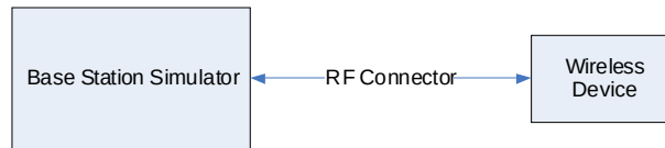
Figure 14-1 Power Measurement Setup
