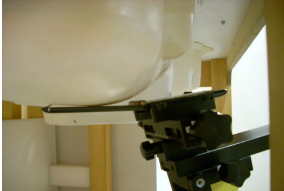
Figure 19-1 SAR Test Setup Photo 1
