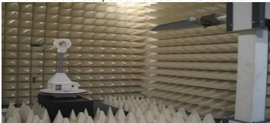
Figure2. Photograph of 3m Fully-Anechoic Chamber
