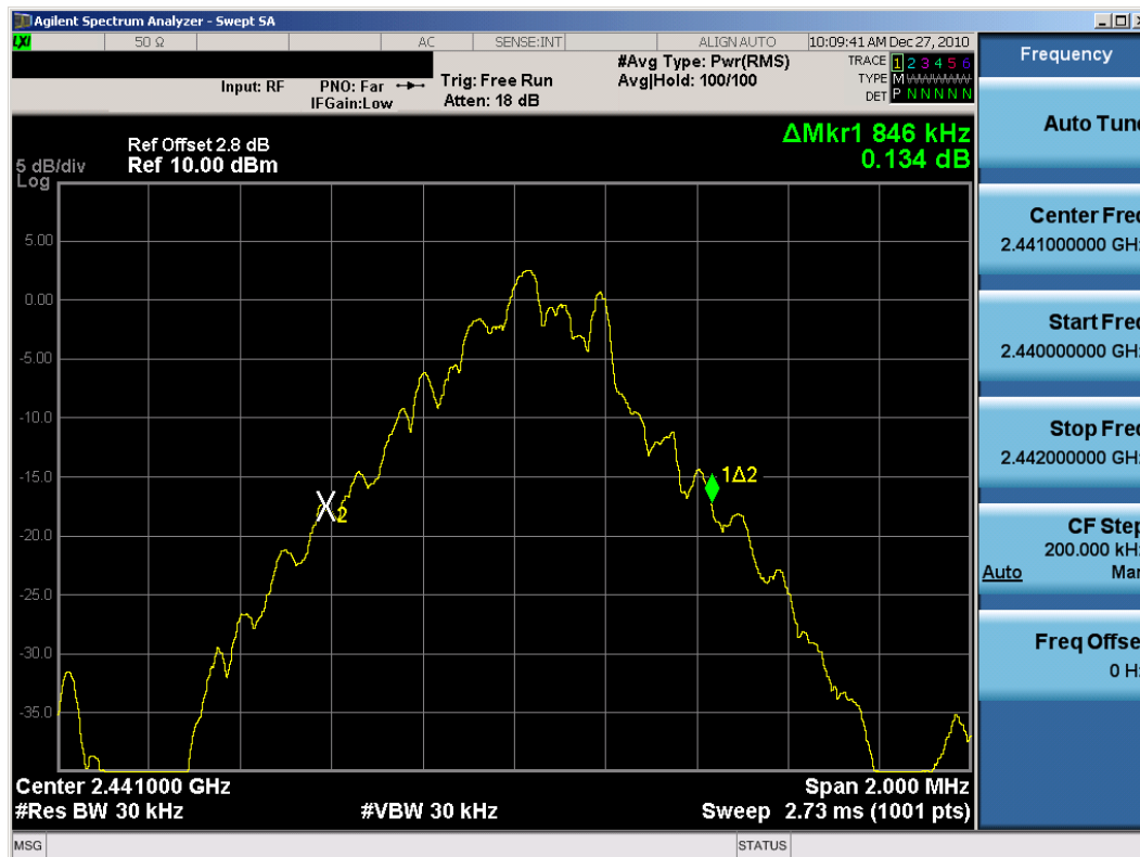
Plot 6-2. 20dB Bandwidth Plot (Bluetooth, 1Mbps – Ch. 39)
