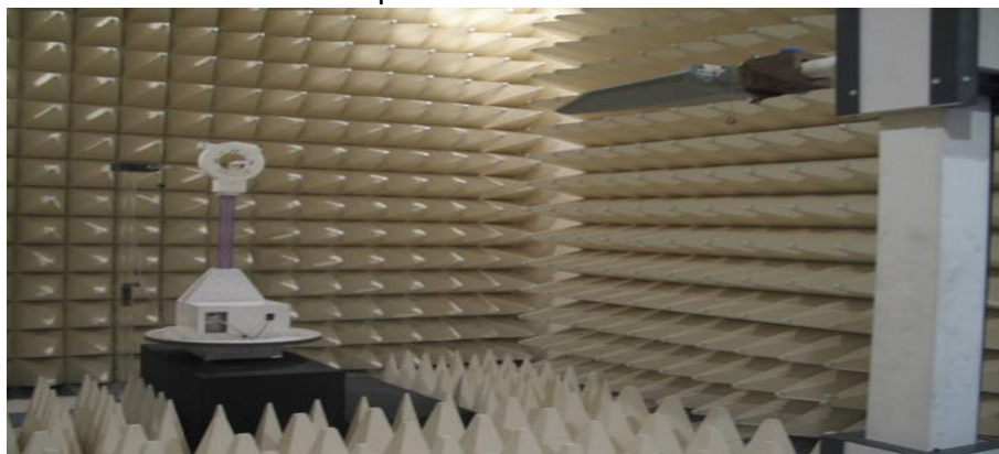
Figure2. Photograph of 3m Fully-Anechoic Chamber
