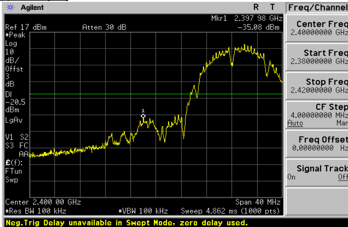
Plot 6-19. Band Edge Plot (802.11b – Ch. 1)
