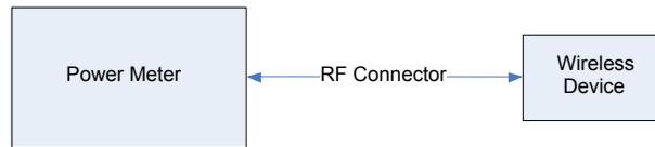
Figure 13-1 Power Measurement Setup
