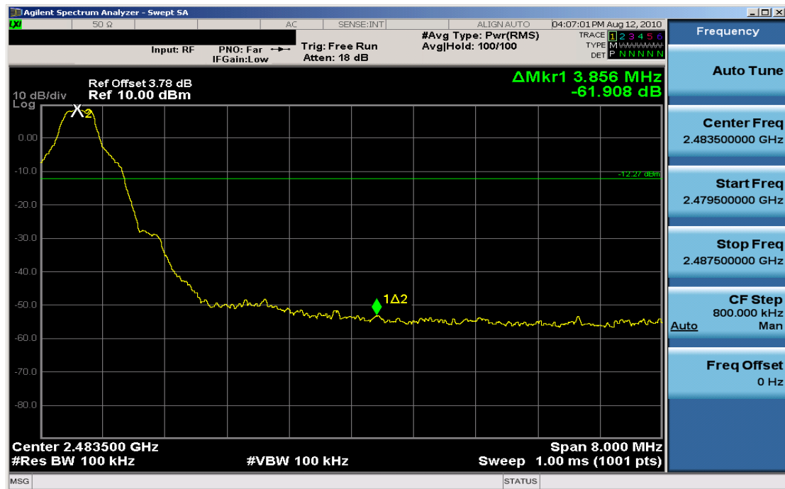
Plot 6-5. Band Edge Plot (Bluetooth – Ch. 78)
