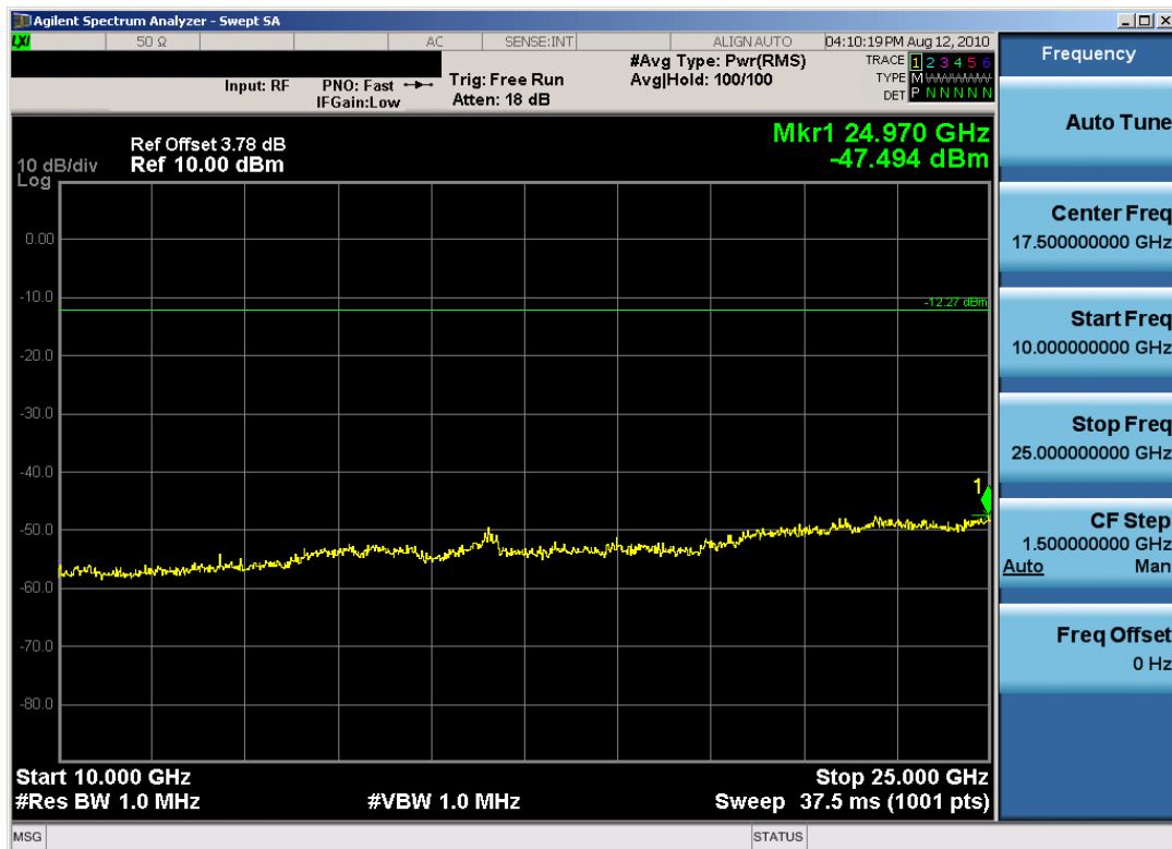
Plot 6-17. Conducted Spurious Plot (Bluetooth – Ch. 78)
