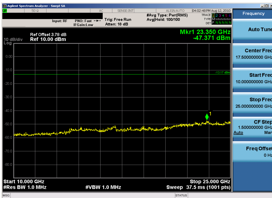
Plot 6-15. Conducted Spurious Plot (Bluetooth – Ch. 39)
