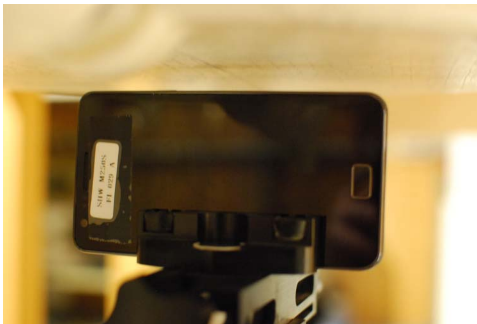
Figure 21-8 SAR Test Setup Photo 8 – Right at 1.0 cm
