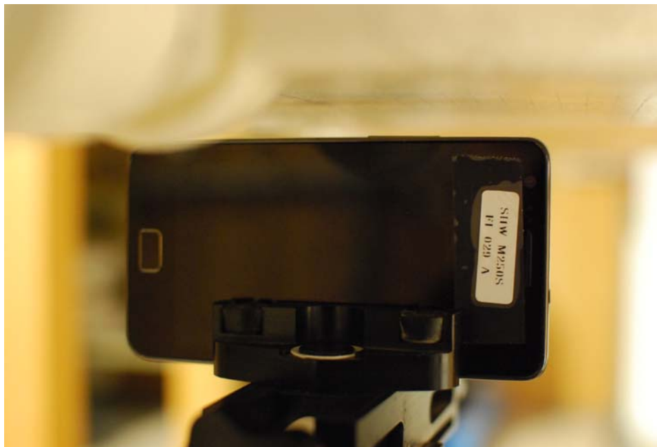
Figure 21-9 SAR Test Setup Photo 9- Left at 1.0 cm
