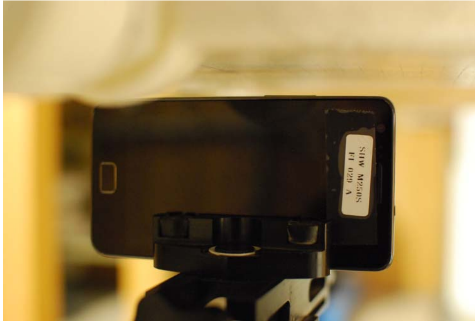
Figure 21-9 SAR Test Setup Photo 9- Left at 1.0 cm
