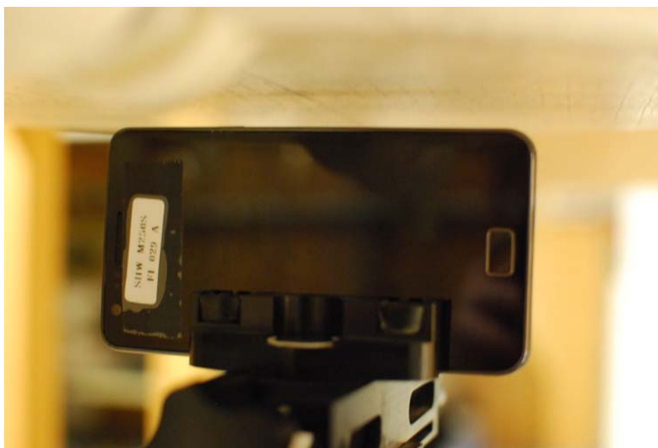
Figure 21-8 SAR Test Setup Photo 8 – Right at 1.0 cm
