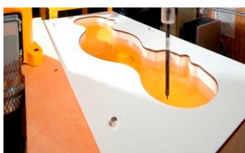
Figure 6-2 SAM Phantom with Simulating Tissue
