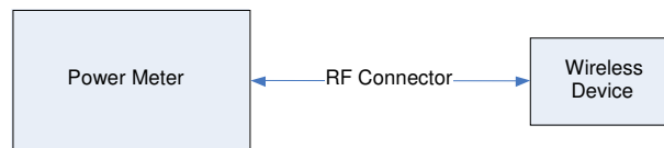
Figure 12-1 Power Measurement Setup
