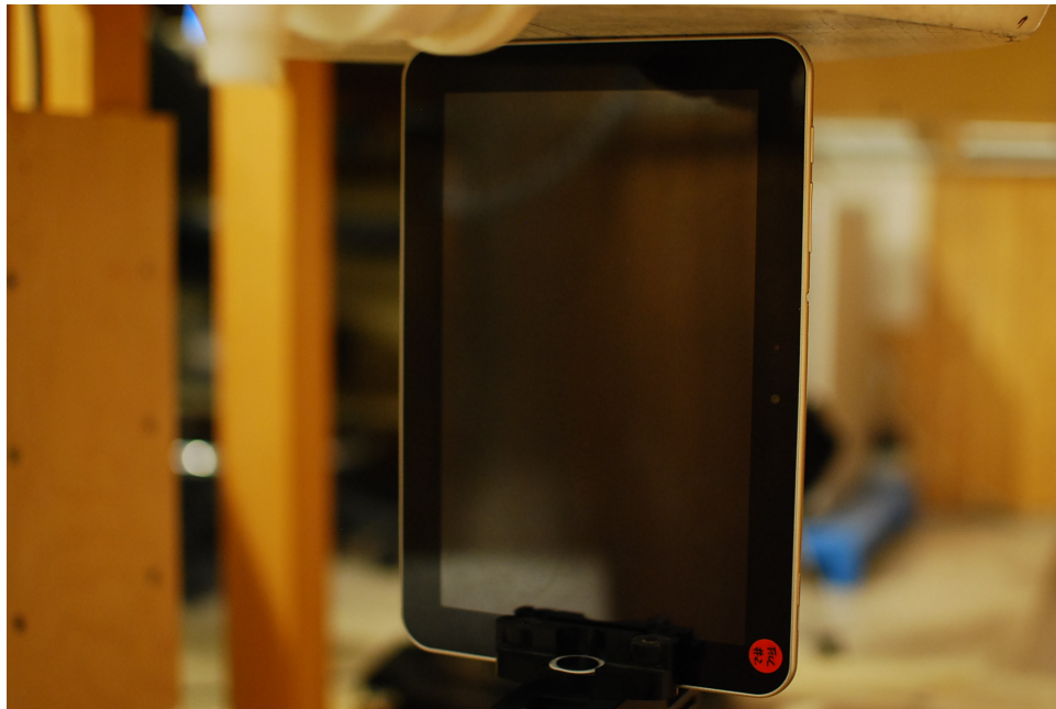
Figure 20-6 SAR Test Setup Photo 6 Photo 6 – Left Edge at 0.0 cm
