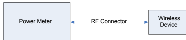
Figure 10-2 Power Measurement Setup
