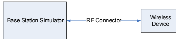
Figure 10-1 Power Measurement Setup
