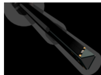
Figure 5-3 Triangular Probe Configuration
