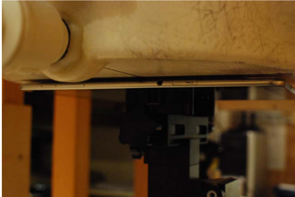
SAR Test Setup Photo 1: Back at 0.0 cm
