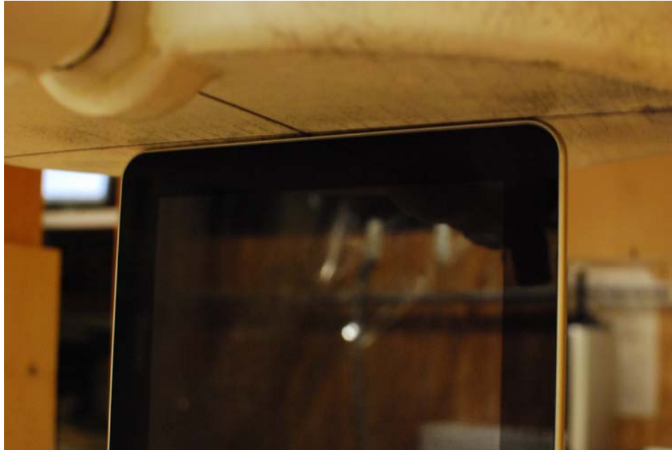
SAR Test Setup Photo 5: Right at 0.0 cm
